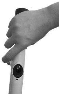
During the time of 10 seconds, the indicator light will flash purple. When the indicator light is fully purple, it means that you are in the setting environment **(your hand must be on the handle all the time when changing settings and the electric wheelbarrow must be in an upright position)**.
